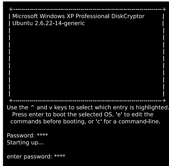
Fig. 20. The "Invisible Man" bypassing both Grub and DiskCryptor authentications by simulating a complex keyboard sequence via "password chaining".
